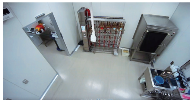
Figure: The new ABSL3 room camera image with Individually Vented Cage systems
