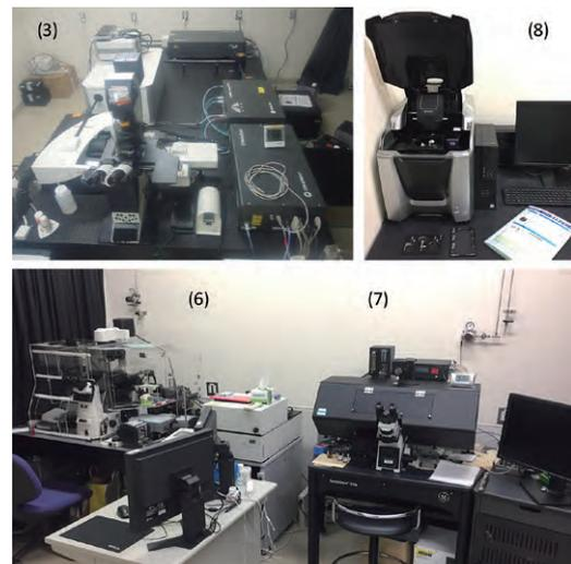
**Photo: Leica SP8 multiphoton microscope (3), Nikon N-SIM/N-STORM super-resolution microscope (6), GE Healthcare DeltaVision Elite system (7), and Keyence BZ-X700 microscope (8).**
