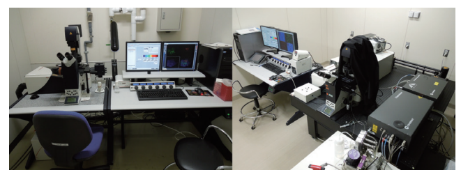
Figure: Left: SP5 confocal microscope (#3). Right: SP5 II two-photon microscope with a femtosecond Ti:Sa laser plus an OPO (#7).
